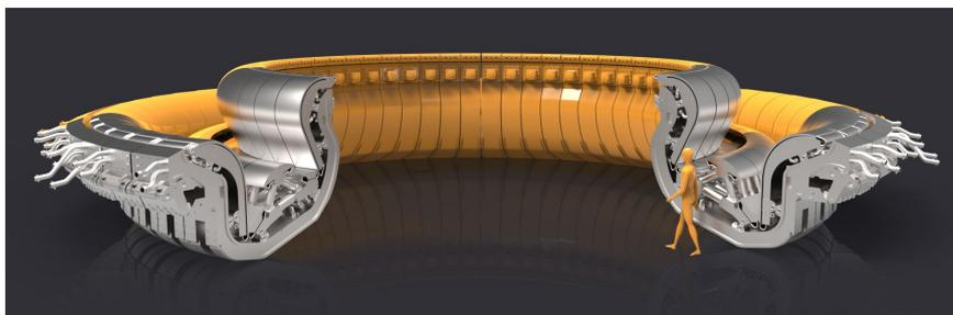
Figure 2.4: ITER divertor, which is placed at the bottom of the vacuum vessel, withstands the highest heat flux from the ITER plasma. (Source of image: Ref. [4])
