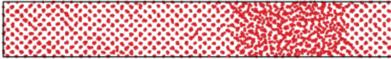
Figure 4.4: Frame 4500, ie. 450 ps into the simulation, of tungsten in a direct simulation, it can be seen that the liquid and the solid phase both still exist. Therefore the melting point could be reached. The system is visualized in OVITO.
